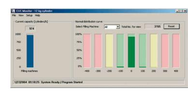
Example of graphic real time display of total filling capacity and filling accuracy
