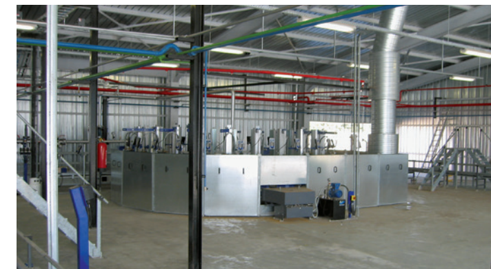
Inside the filling hall, the new electronic EFC/24 filling carousel with 24 UFM's
