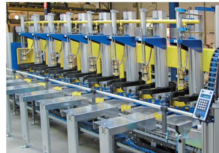
Fully automatic in-line evacuation system
