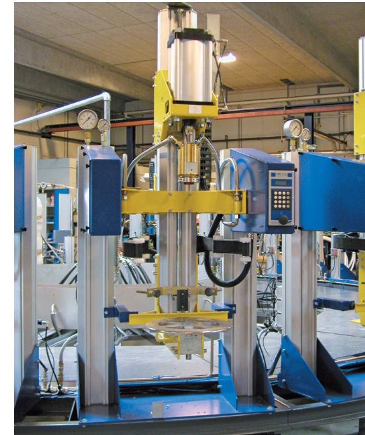
Pressure testing unit on PTC-20 pressure testing carousel
